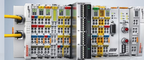
EtherCAT I/Os: Broad I/O spectrum in IP20 and IP67
