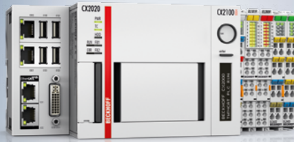
Embedded PCs: IPCs with integrated I/O level
